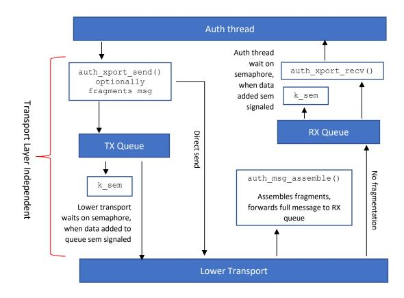
The Bluetooth Central Authentication sample (see samples/authentication/bluetooth/central\_auth) provides a good example to drill deeper into the transport layer interface and how Bluetooth is "hooked up" to ZAUTH. The **GREEN** boxes are Bluetooth transport specific.
